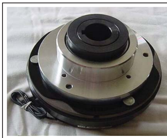
Replacing the existing engine cooler drive sheave with a clutch-pulley system that disengages the cooler drive when the evaporative system is operating makes additional horsepower available for compression.
